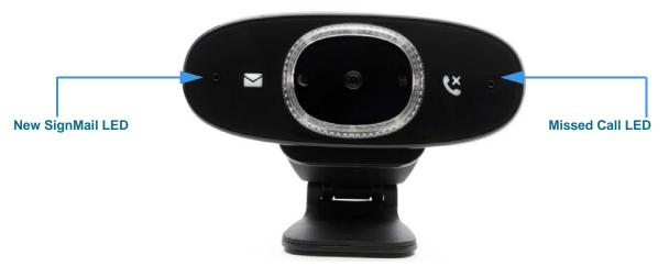
The "Camera Notifications" feature are the two icons printed on the front surface of the camera and two LEDs located next to the icons. If you like, you can turn off this feature off so that the LEDs will not light up when you receive new SignMails or missed calls.
